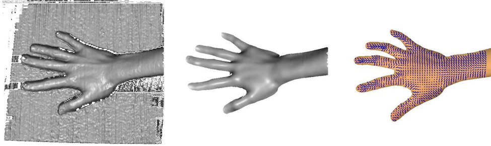
Figure 3: Result of depth processing. From left to right: raw input depth from the hand video, thresholded and smoothed depth, needle map (computed surface normal distribution). Note that both depth maps are rendered with a light source for clarity.
